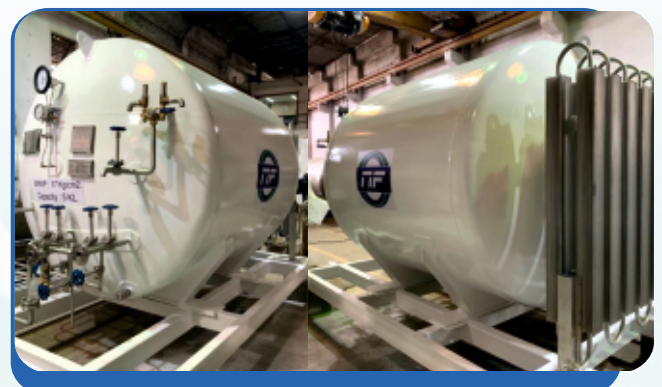
05KL CRYOGENIC STORAGE TANK
